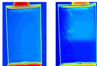
**Figure 2.** Image of a single PRESAGE® dosimeter prior to irradiation (left) and 24 hours after irradiation by a proton beam (right). Images taken from the DMOS reconstruction software.
