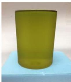
**Figure 1.** A PRESAGE® dosimeter formulated for high-LET dosimetry.
